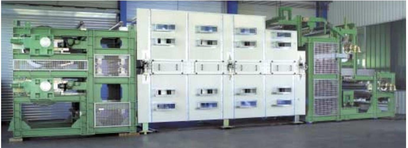
A typical example of the recently developed double belt press for low pressure applications for the production of fibre compound
