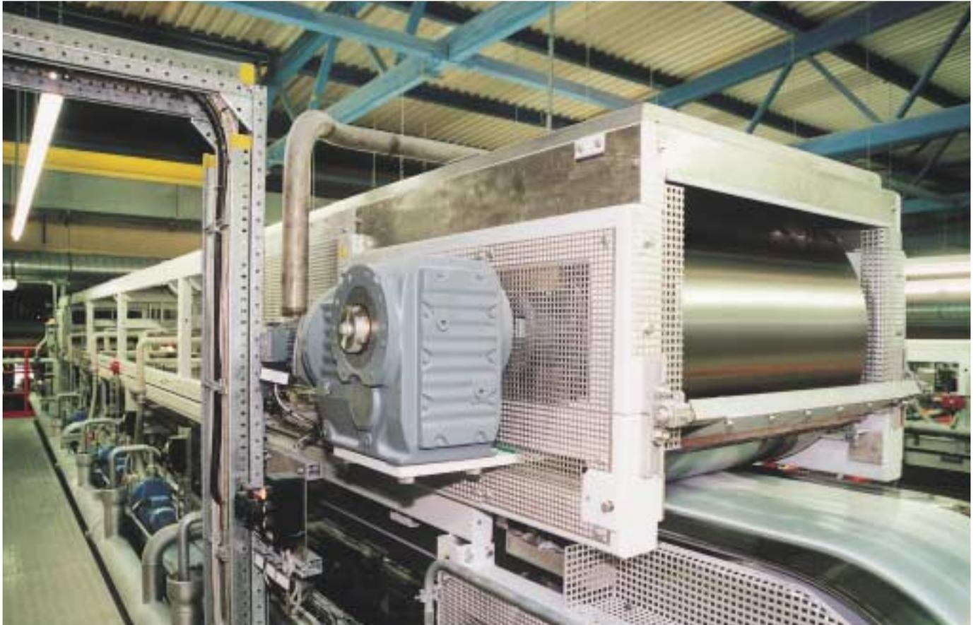
Double belt cooler for continuous production of silicon
